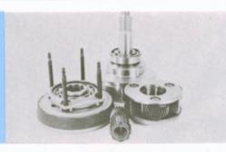
Inspect gears and bearings. Inspect bushing in sunwheel.
