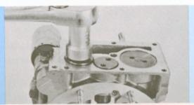
Remove plug, large piston, and spring. (52,54,50)
