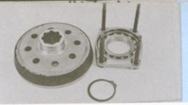
Disassemble sliding member, bearing, and retainer.
