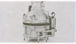
Install nuts and washers holding casings together. (91,90)
