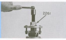
Pull flange off output shaft. Press output shaft out of rear casing. (116,110)
