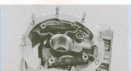
Install bridge pieces, Lock washers and nuts or self locking nuts. If installed, bend washers to lock nuts. (3,14,1)
