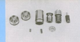
Inspect pistons, valves, 25 pump plunger, bodies, and cylinders. Inspect springs for damage. (23,42,54,66,64,41, 50,44,58,61)
