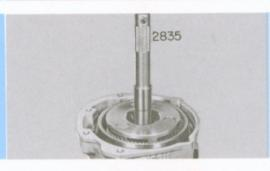
Install planet carrier in shaft. Line up splines. (73)
