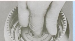
Install thrust washer and clutch in shaft. (85,88)
