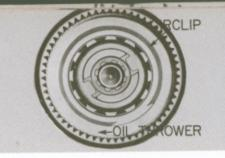
Remove circlip, oil thrower, uni-directional clutch, and thrust washer from output shaft. (87,86,88,85)
