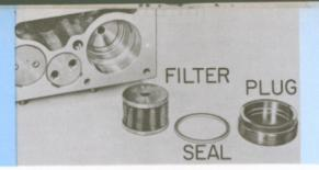
Remove plug, fine filter, and seal. (70,68,69)
