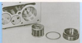
Remove, clean, and install plug, filter, and seal. (70,68,69)
